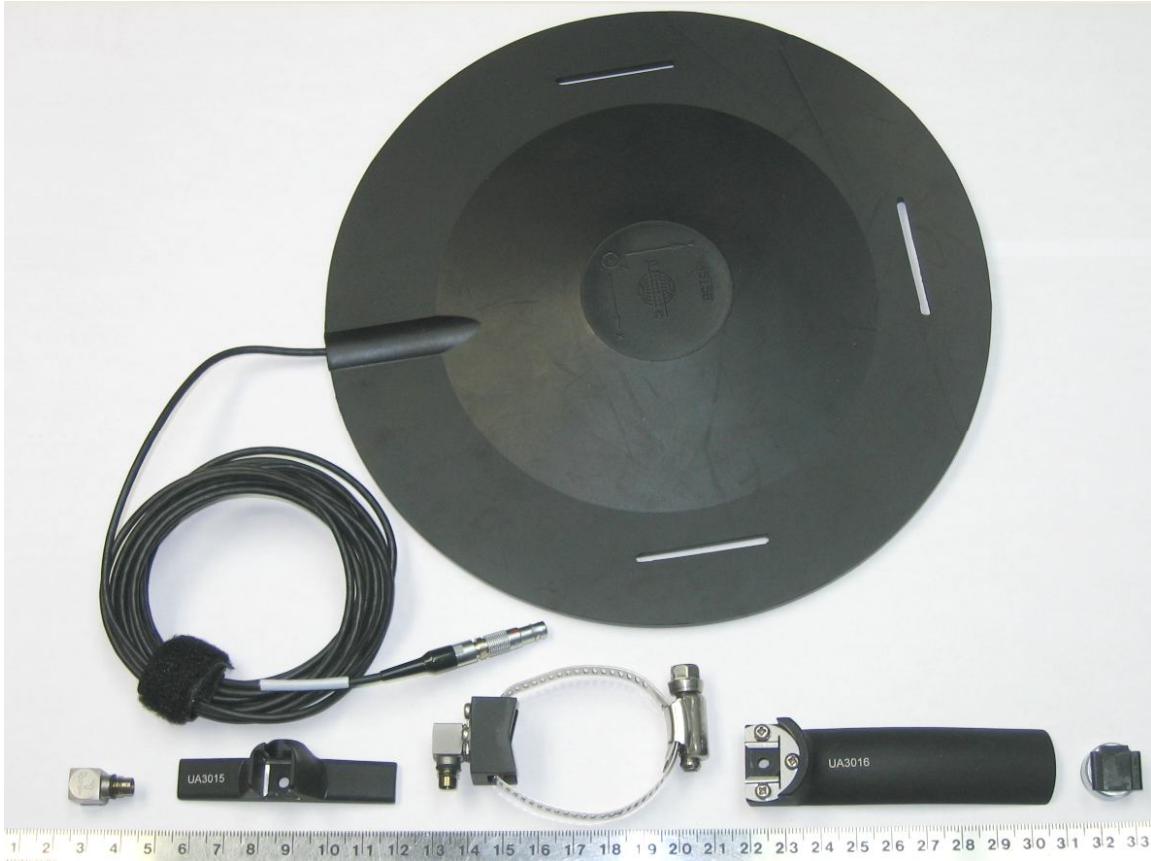
Figure 4: Example of a tri-axial accelerometer and mounting accessories
